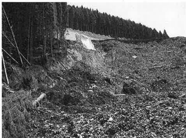
Photo 2 Head scarp exposing black and reddish brown clayey soil layers showing failure plane with striations. Note, debris from the embankment slides consisted of fragmented sandstone and clayey soil. The soil cover was less than 1m thick and the sliding exposed the underlying bedrock
